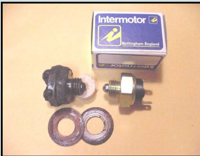
New and used interrupter switches—note the wear in the unit on the left. Also shown are the fiber washers.
